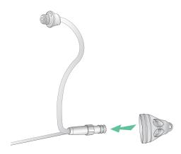
To remove the dome, grasp the dome between the thumb and forefinger and pull it off the slim tube HE.
