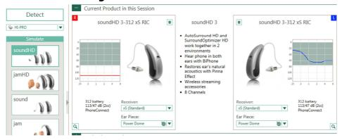
Make selections on the Acoustics & Accessories screens as appropriate. Run the Feedback manager if desired, but it is only necessary to run it for the better (in this case Left) ear.
